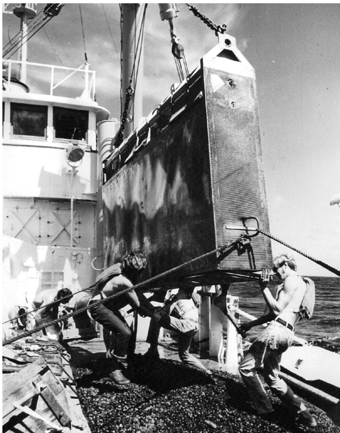
Using dredges, some companies managed to recover manganese nodules from the deep sea, 5,000 m below.
